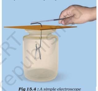
The aluminium foil strips receive the same charge from the charged refill through the paper clip (remember that metals are good conductors of electricity). The strips carrying similar charges repel each other and they become wide open. Such a device can be used to test whether an object is carrying charge or not. This device is known as **electroscope**.
