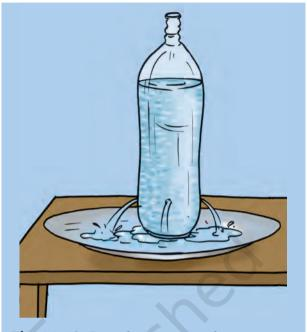
**Fig. 11.16:** Liquids exert equal pressure at the same depth
