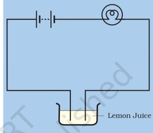
**Fig. 14.2 :** Testing conduction of electricity in lemon juice or vinegar
