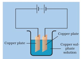
**Fig.14.7**: A simple circuit showing electroplating
