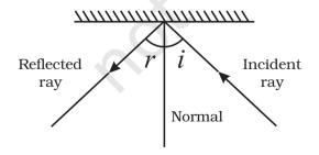
**Fig. 16.3:** Angle of incidence and angle of reflection
